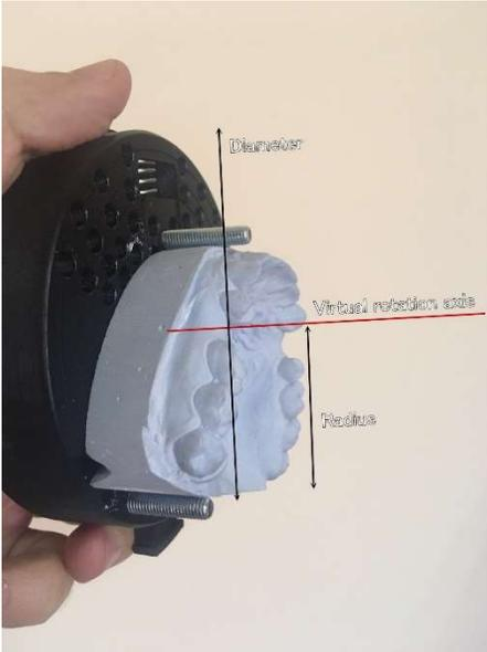
This software parameter specifies the object extension relative to the mount's rotation axis, or mount center (not the center of the part). To measure this value take the imaginary rotation axis of the mount and find the point on the object furthest away from this rotation axis. In this way, you can get the radius of the object relative to the rotation axis. Then multiply this value by 2 to get the *diameter*.
