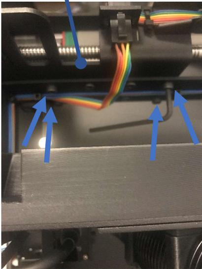
1. The instrument vertical stage needs to be raised up to allow easier access to the mount screws. See Software Installation Section, or the vertical lead screw can be turned by hand to raise the vertical stage.
