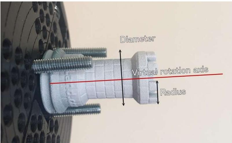
Suppose you have an object that doesn't have symmetry according to the rotation axis. In this case, you do the same, find the farthest point, and measure the distance to the rotation axis as shown below.
