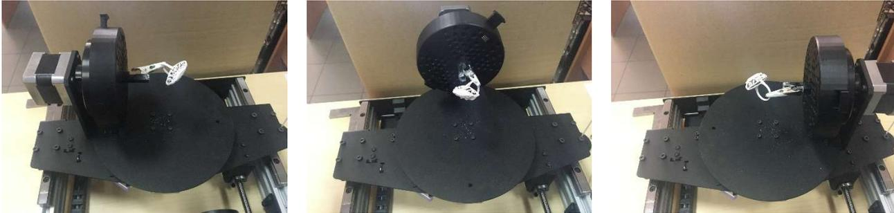
The vertical rotations in software corresponds to the table positioned vertically. If you specify "N" vertical rotations then the program take measurements every  $360/N$  degrees. For example, if you specify 8 vertical rotations then the scanner will make 8 scans and rotate the vertical table 45 degrees ( $360/8=45$ ) for each scan as shown below.
