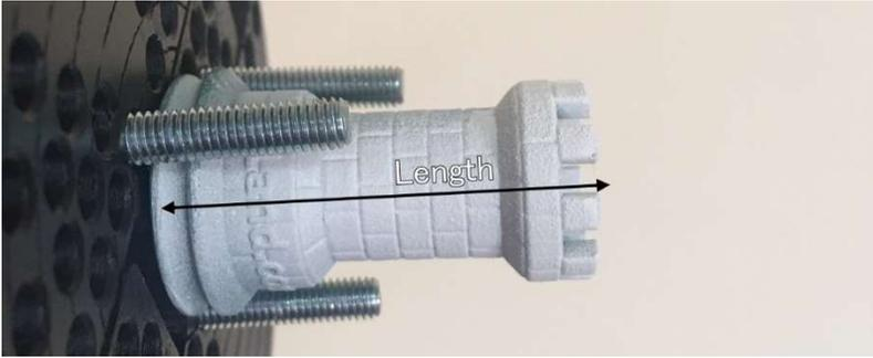
The length software parameter specifies the length of the object along the rotation axis. You can specify only part of the object that you want to scan by selecting a shorter length value.
